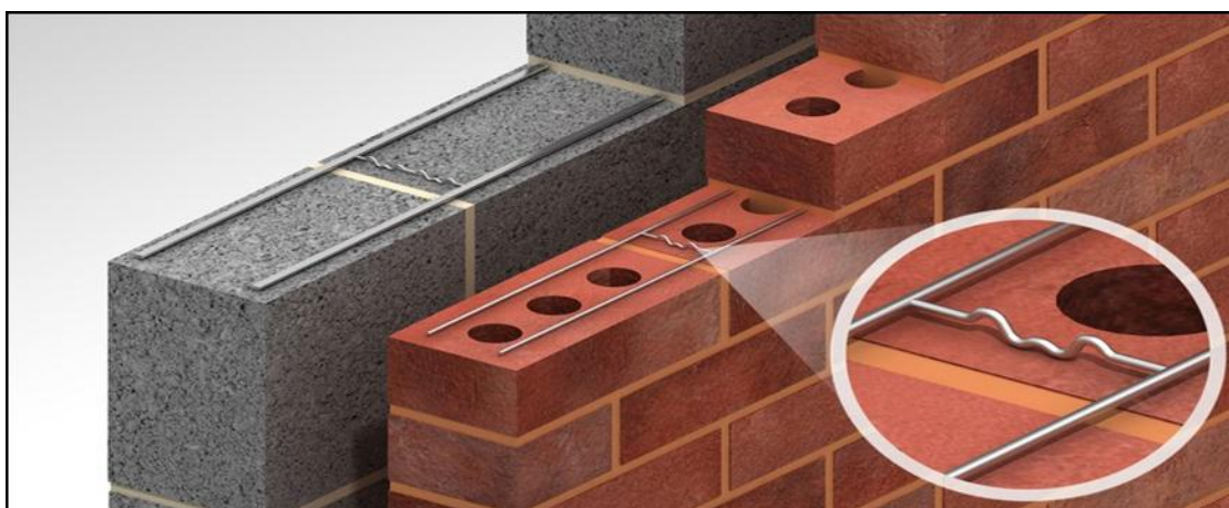
Above: Example of cavity wall construction including insulation slabs installed in a similar fashion to that specified for the PPP1 schools.
